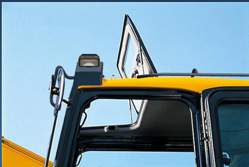
Standard openable skylight
