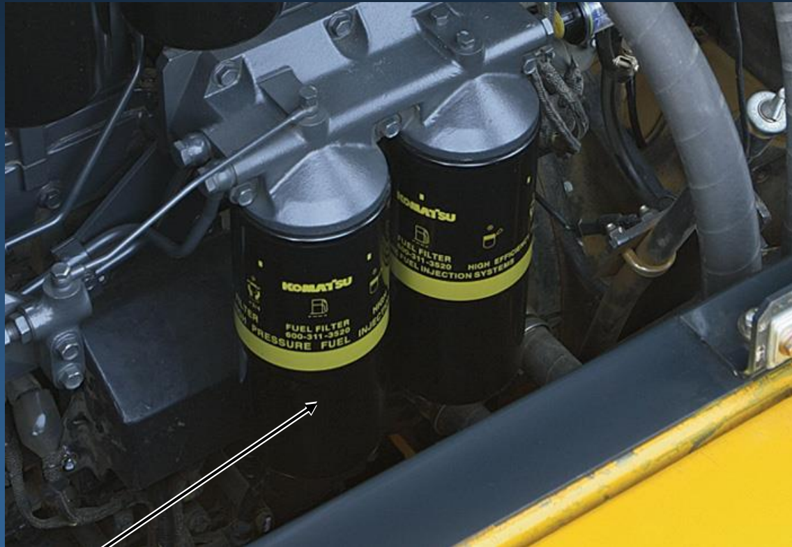
Additional fuel main-filter
